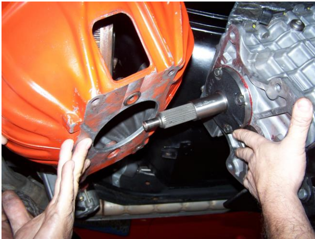
CLUTCH FORK SHOULD ALREADY BE INSTALLED AT THIS POINT, REMOVED FOR CLARITY IN PHOTO
