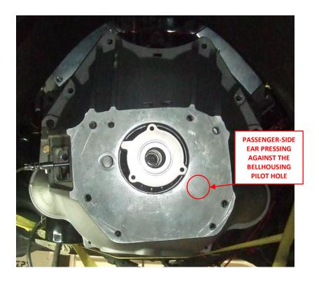
7. Align the stud with the bearing upper mounting ear hole and install the transmission as shown below. Once the input shaft enters the hydraulic bearing, the bearing will align itself with the bellhousing pilot hole and slide into place.
