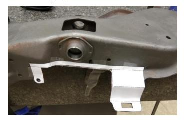
3. Attach bracket to the clutch pedal arm using the (2) 5/16-18 x 1" bolts and nuts provided.
