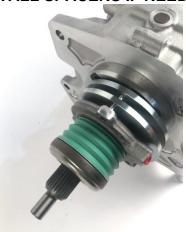
If your cushion measurement is **LESS** than 1/8", you will need a boundaring apace. To move the transmission and CSC further away from the engine block. The spacer is 1/4" thick, and gets sandwiched in between the bellhousing and the transmission. You can only use one bellhousing spacer. If you need more than 1/4" to get your cushion within specs, you may have to resurface the flywheel, change to a thinner flywheel, or change to a different clutch.
