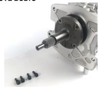
3. TKO,TKX: Remove the front bearing retainer by tapping lightly with a mallet to break it free. TKO/TKX: Be sure to keep pressure on the input shaft to prevent it from moving. This is the reason for tilting the transmission in step one. It is very important to not let the input shaft move, otherwise the transmission may need complete disassembly. (FIG. B).
