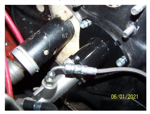
6. From passenger compartment, assemble backing plate, lock washer and nuts. Align master cylinder, then tighten bolts to 15 ft.-lbs.
