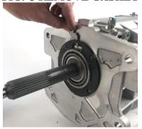
5. **TKO/TKX**: If the bearing race came out with the bearing retainer, remove it from the old bearing retainer and insert it into the transmission, taking care not to lose or damage the input shaft shims that are between the bearing retainer and the bearing race (FIG. D). If the race stayed in the transmission, be sure to remove the shims from inside the old bearing retainer. Clean old sealant from the front of the transmission case using a razor blade scraper.
