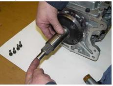
4. **TKX:** Save the gasket from the bearing retainer. NOTE: The gasket must be used in the endplay measurement as the gasket itself is 0.010in thick.
