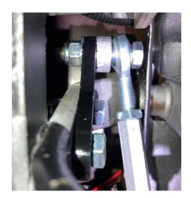
6. **DO NOT** depress the pedal any more than necessary before fluid is added to the system. **DOT 4 BRAKE FLUID STRONGLY RECOMMENDED.**
