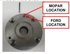
FIG. G RETAINER PROPERLY INSTALLED
