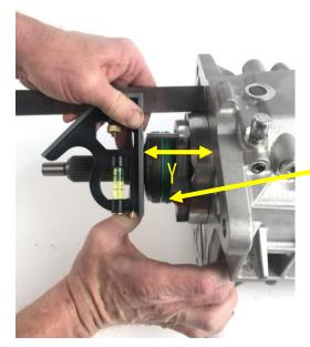
MEASURE FROM THE FRONT OF THE TRANSMISSION CASE TO THE SURFACE OF THE FULLY COLLAPSED BEARING FOR YOUR "Y" DIMENSION.
