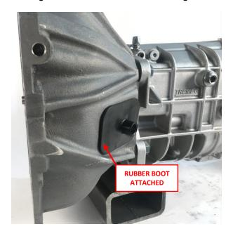
3. Insert hydraulic line from outside of bellhousing with the bleeder pointing down and start threading into the throw-out bearing.
