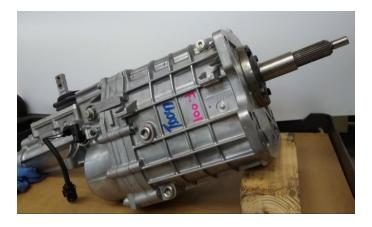
2. **TKO,TKX:** Remove four (4) bolts holding the front bearing retainer to the transmission (FIG. A).
