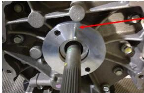
Install with the locating stud at the 12 o'clock position. Tighten (2) 6mm x1.0 screws to 12 Nm or 106 in lbs.
