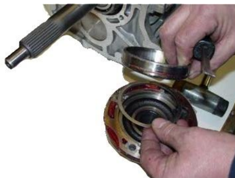
FIG. C (TKO/TKX ONLY) REMOVE BEARING RACE AND SHIMS
