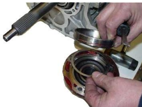
FIG. C (TKO/TKX ONLY) REMOVE BEARING RACE AND SHIMS
