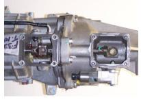
18) There are two different sized rear shifter opening cover plates included in your kit. Select the appropriate size cover for your transmission. Apply a bead of gasket sealant around the shifter opening on the transmission, and install the new rear cover using the shorter bolts supplied with kit. If desired, affix the "STX" shifter badge to the new cover plate.
