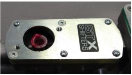
5. Install shifter gasket, and shift tower assembly to shifter baseplate. Use the two 5/16-18 x 2in, apply some rtv to the threads, and torque to 12-16 lb-ft.
