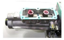
4. Install shifter baseplate using the 6 bolts provided be sure to use the 2 flat screws in the countersunk locations. Tighten bolts to 6-11 lb-ft torque.
