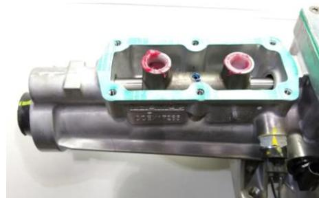
4. Install shifter reusing the 6 bolts from the old shifter. Tighten bolts to 6-11 lb-ft torque.
