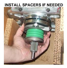
\*\*\*\*\* NOTE: The bearing cushion will also need to be re-measured and recalculated after resurfacing or replacing the flywheel, or changing the bellhousing, engine, or clutch. Different clutches have different stack-up heights, and a scattershield is often deeper than a factory GM bellhousing.
