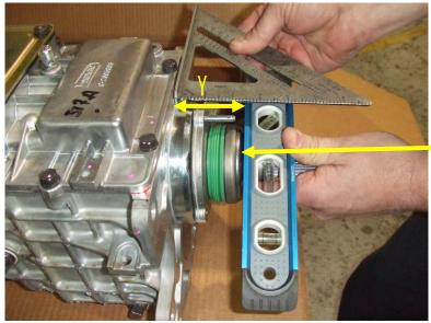
MEASURE FROM THE FRONT OF THE TRANSMISSION CASE TO THE SURFACE OF THE FULLY COLLAPSED BEARING FOR YOUR "Y" DIMENSION.
