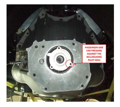
6. Align the stud with the bearing upper mounting ear hole and install the transmission as shown below. Once the input shaft enters the hydraulic bearing, the bearing will align itself with the bellhousing pilot hole and slide into place.
