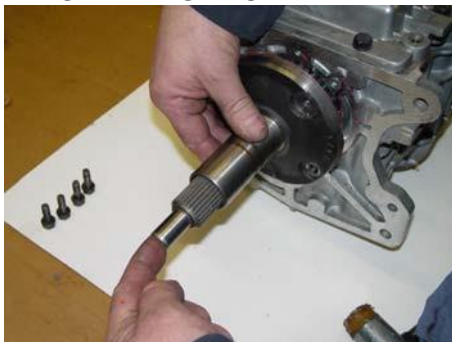
FIG. B REMOVE OLD RETAINER
