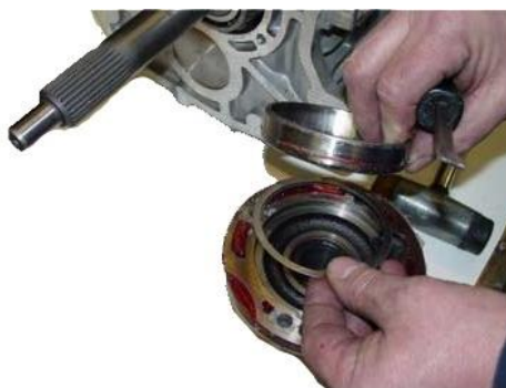
FIG. C (TKO/TKX ONLY) REMOVE BEARING RACE AND SHIMS
