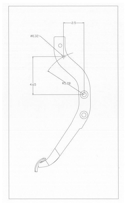
**Clutch Pedal Lower Section Drawing**
