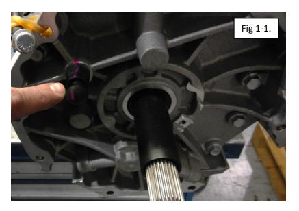
2. Remove the detent assembly from the top of the front cover of the magnum.
