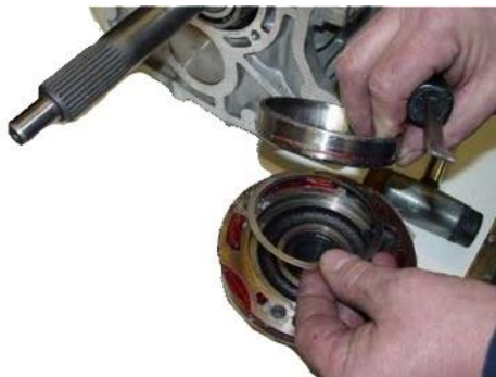
FIG. C (TKO/TKX ONLY) REMOVE BEARING RACE AND SHIMS
