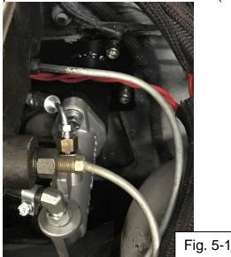
Use caution not to over tighten and break fittings. DO NOT depress the pedal any more than necessary before fluid is added to the system.
