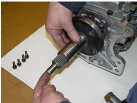
FIG. B REMOVE OLD RETAINER
