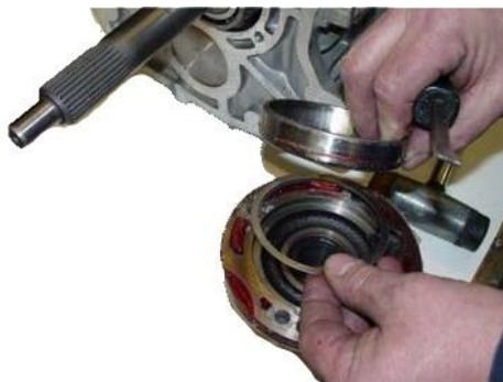
FIG. C (TKO/TKX ONLY) REMOVE BEARING RACE AND SHIMS
