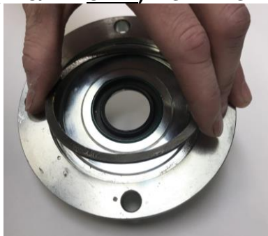
FIG. D (TKO/TKX ONLY) INSTALL SHIMS IN RETAINER
