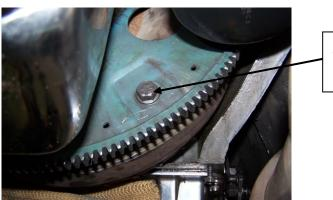
REMOVE TORQUE CONVERTER BOLTS
