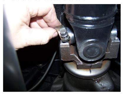
Pull slip yoke out to meet the front u-joint and attach.
