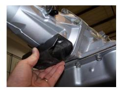
o Never install a solid isolator mount - this could cause case to break.
