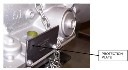
o Install isolator mount to bottom of transmission tailhousing using hardware pack hwg-pack h.
