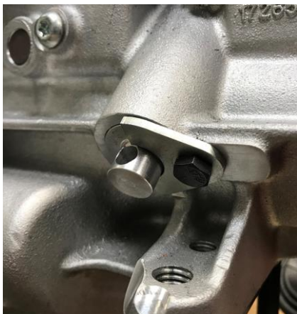
MECHANICAL SPEEDOMETER PORT
