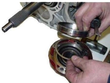
6. **TKO/TKX:** Place shims into new bearing retainer, using petroleum jelly to hold them in place. Install the thickest shim closest to the bearing race.
