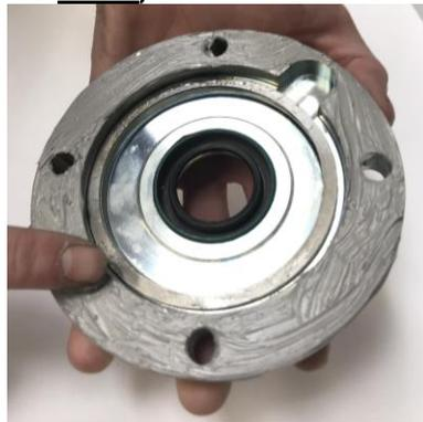
11. **ALL:** Position the new bearing retainer so that the locating stud is at the top (12 o'clock) position and attach it to the transmission using four (4) socket head cap screws (FIG. F & FIG. G). Torque the socket head cap screws to 12-16 lb.-ft. in an "X" pattern.
