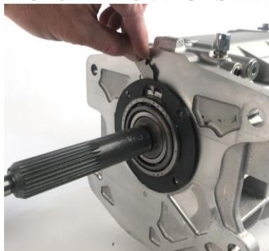
5. **TKO/TKX:** If the bearing race came out with the bearing retainer, remove it from the old bearing retainer and insert it into the transmission, taking care not to lose or damage the input shaft shims that are between the bearing retainer and the bearing race (FIG. D). If the race stayed in the transmission, be sure to remove the shims from inside the old bearing retainer. Clean old sealant from the front of the transmission case using a razor blade scraper.
