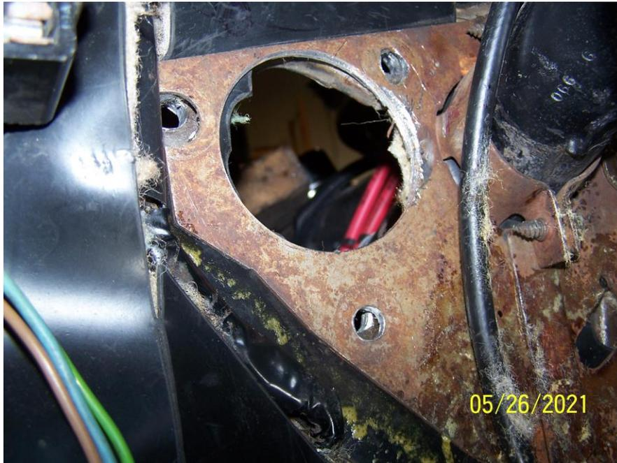
3. The mount block is installed using factory firewall welded nut location (3). Drill out nut threads to 3/8" hole for attaching mount using kit supplied 5/16" machine screws. Additionally, the firewall has a lip that will need to be trimmed or flattened for the mount block to sit flush.
