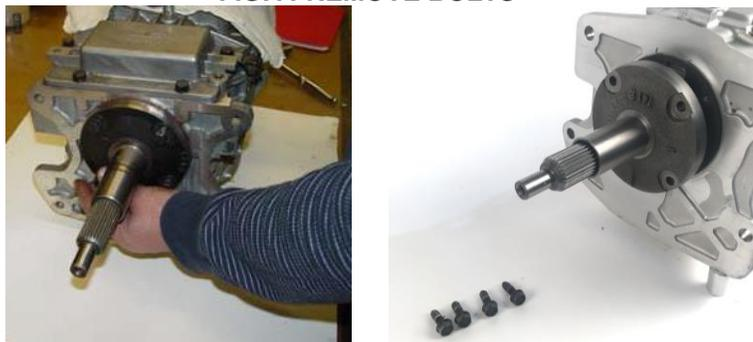
3. **TKO,TKX:** Remove the front bearing retainer by tapping lightly with a mallet to break it free.
