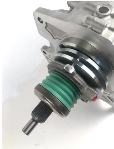
If your cushion measurement is **LESS** than 1/8", you will need a bellhousing spacer to move the transmission and CSC further away from the engine block. The spacer is 1/4" thick, and gets sandwiched in between the bellhousing and the transmission. You can only use one bellhousing spacer. If you need more than 1/4" to get your cushion within specs, you may have to resurface the flywheel, change to a thinner flywheel, or change to a different clutch.
