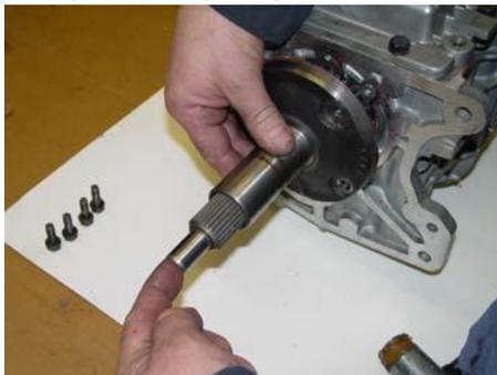
4. **TKX:** Save the gasket from the bearing retainer. NOTE: The gasket must be used in the endplay measurement as the gasket itself is 0.010in thick.
