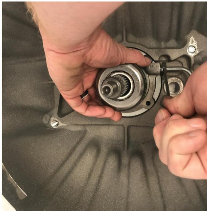
5. Remove the bellhousing with the hydraulic bearing and assembled line attached.
