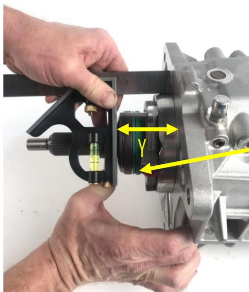
**MEASURE FROM THE FRONT OF THE TRANSMISSION CASE TO THE SURFACE OF THE FULLY COLLAPSED BEARING FOR YOUR "Y" DIMENSION.**
