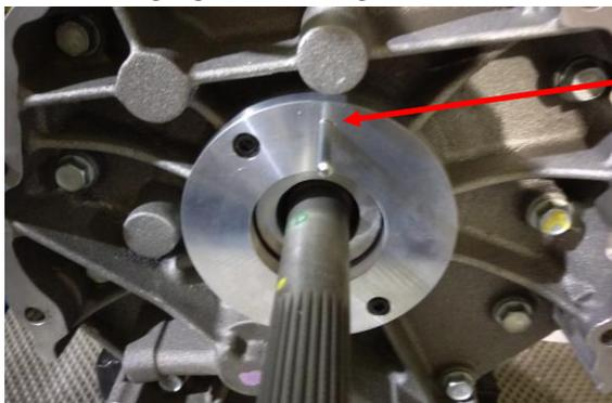
Install with the locating stud at the 12 o'clock position. Tighten (2) 6mm x1.0 screws to 12 Nm or 106 in lbs.
