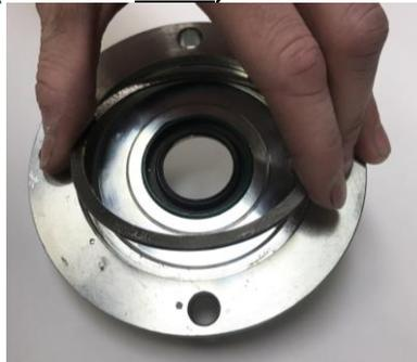
7. **TKO/TKX:** Position the new bearing retainer without sealer so that the locating stud is at the top (12 o'clock) position and attach it to the transmission using four (4) socket head cap screws (FIG. F & FIG. G). Torque the socket head cap screws to 12-16 lb.-ft. in an "X" pattern.
