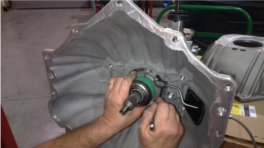
4. Remove the bellhousing with the hydraulic bearing and assembled line attached.
