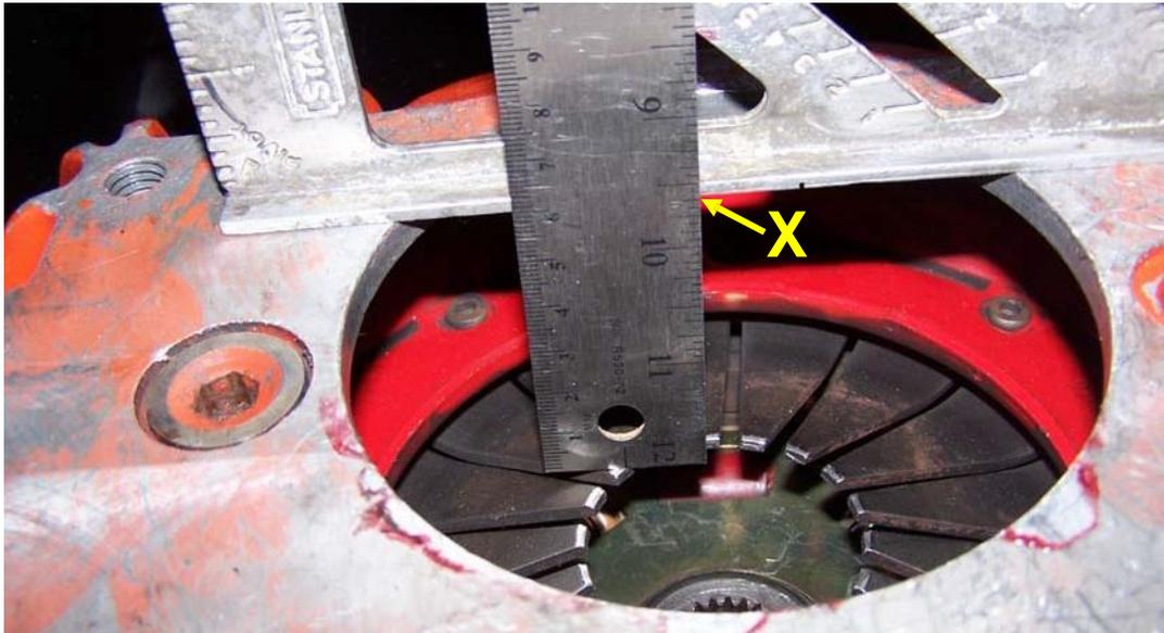
3. Next, with the slave cylinder mounted on the transmission, compress the CSC against its internal spring pressure back towards the transmission. With the CSC compressed to its internal stop (completely bottomed out), hold a straight edge across the face of the throw-out bearing and measure the distance from the face of the bearing to the bellhousing mounting face of the transmission. Record this dimension ( **Y** ).
