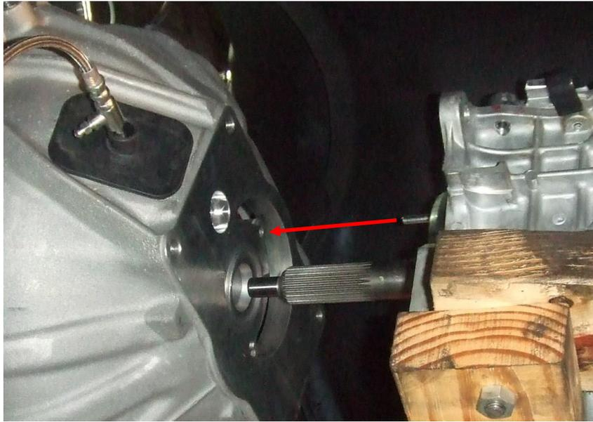
**NOTE: You may have to slightly twist the transmission left or right in order to align the stud with the hydraulic bearing. If you are not using a transmission jack, obtaining assistance from another person might be needed.**
