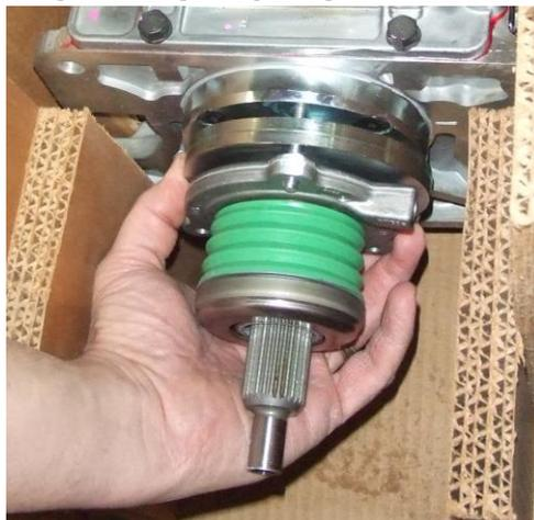
**\*\*\*\*\* NOTE:** The bearing cushion will also need to be re-measured and recalculated after **resurfacing or replacing the flywheel, or changing the bellhousing, engine, or clutch.** Different clutches have different stack-up heights, and a scattershield is often deeper than a factory GM bellhousing.
