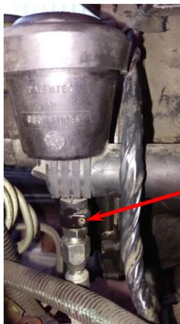
Pin to be removed. It may be necessary to remove the master from the vehicle to remove the pin.
